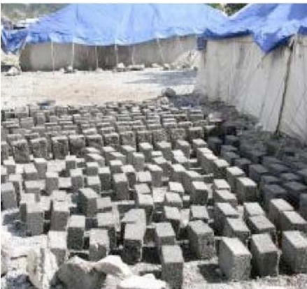
Building blocks for reconstruction purposes which can be produced from recycled building waste, Pakistan.
